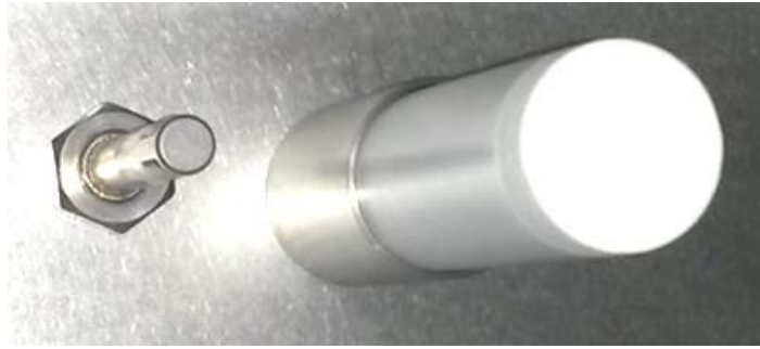
Figure 13: Plugged-in CO 2 sensor (right) and gas mixing head for CO 2
